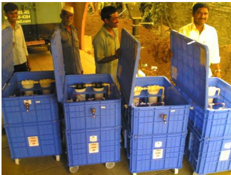
Madhu Tara that works on hand pump and also with electricity (100 LPH)
