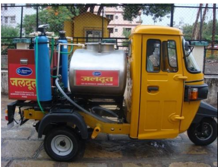
Jal Doot a mobile water filtration system that goes house to house for delivering water in villages
